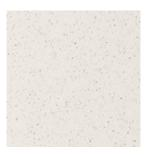
The feldspar particles contained in the quartz material can become visible after surface treatment as black and/or white dots, small, formless areas created by clump building during the mixing process and occasionally appears on the surface.
