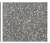
Colour differences caused by variations in material quality can occur by products with inlays such as forms of hard rock grit, mother of pearl, silicon and chipped mirror glass particles. Isolated breakouts and/or flaking of up to 2–3 mm in diameter are technically unavoidable and must be tolerated by the customer.
